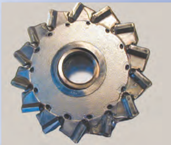
Wear protected cutter hub
