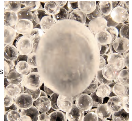
PLA pellets cut with a Gala Underwater Pelletizer
