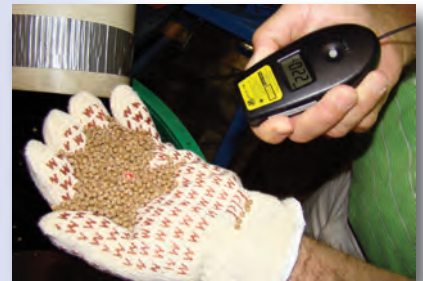
PP Wood Fiber cut with a Gala Pelletizer
