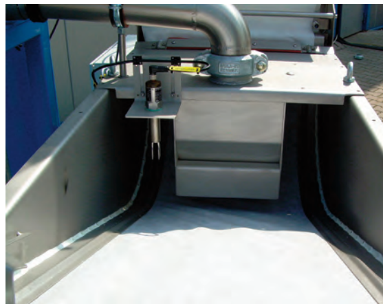
Tempered water system tank with band filter medium to remove down to 20 µm particles
