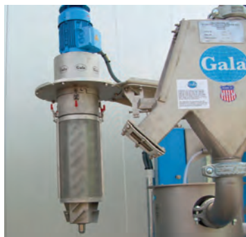
TWS 500-BF2 with band filter in tank
