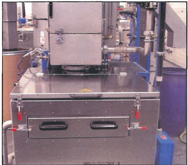
Euro Model CIS, with insulated tank for high temperature applications.
