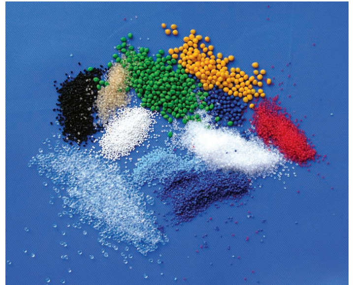
An assortment of micropellets, minipellets and standard 3 mm pellets – all produced using Gala technology and equipment.
