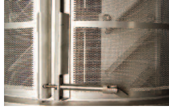
Perforated Screen used for most dryer applications
