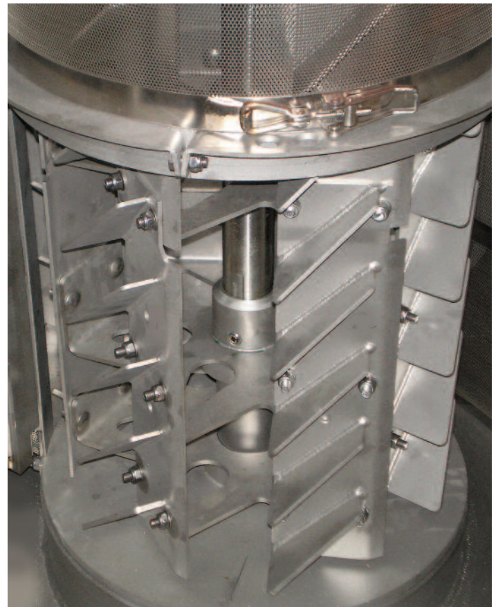
Rotor area of a 2016 BF Dryer
