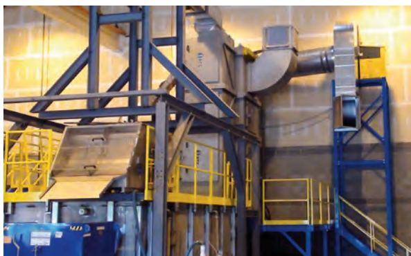
Dryer Model 100 at Gala's Dryer Test Facility for rates up to 100 t/h
