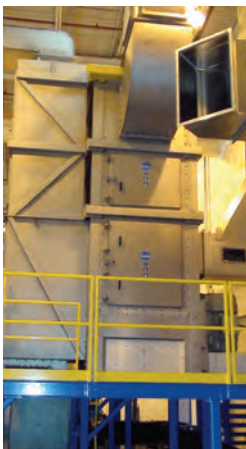
Dryer Model 100 at Gala's Dryer Test Facility for rates up to 100 t/h
