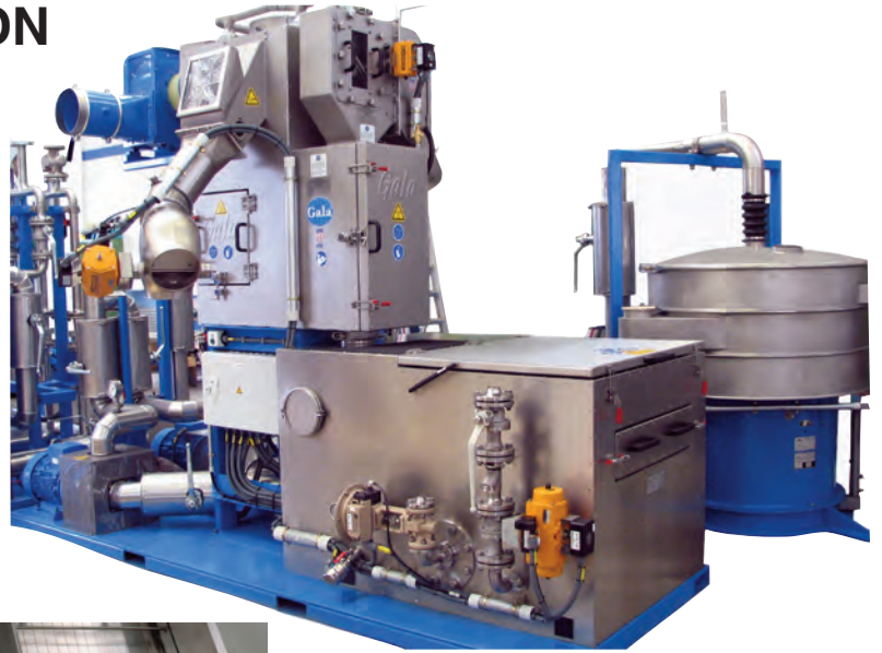
TWS 70 Water System with Dynamic Water Filtration, insulated version
