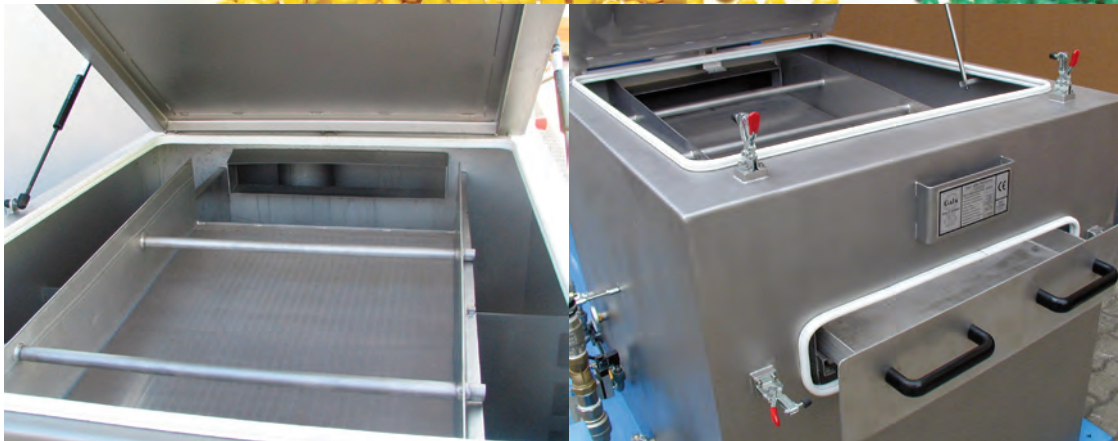
Tempered water system tank with integrated fines removal screen system to remove down to 300 µm particles
